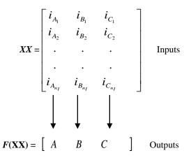
The input data, consisting of normalized absolute values of three pre-fault and four post-fault samples of each of the three phase currents,  $i_A$ ,  $i_B$ ,  $i_C$  are presented to each of the two ANNs used for fault classification, in the form of multiple input vectors as shown above. This type of batching operation is more efficient than the case when inputs are presented in the form of a single vector [30].
