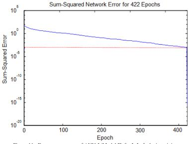
Figure 11: Error convergence of ANN-I (Model II) for L-L faults in training
