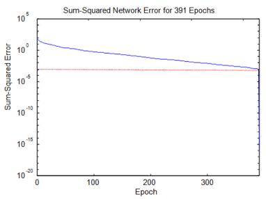
Figure 12: Error convergence of ANN-II (Model II) for L-L faults in training
